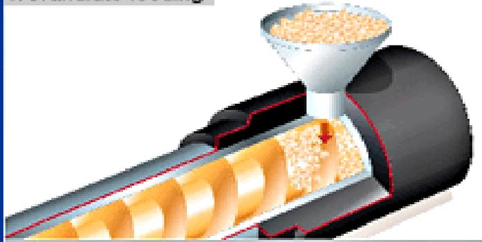
The rotating screw draws in the granulate from the material hopper and transports it in the direction of the screw tip.
